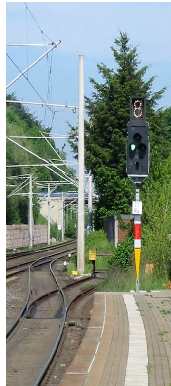
Figure 3: German main line railway signal with speed indication number showing maximum speed of 80km/h.
