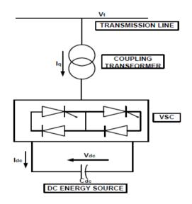
Fig.6 Structure of STATCOM
