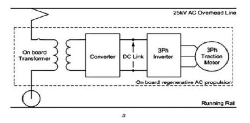
Fig.4. Block diagram of AC locomotive
