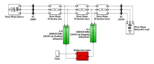
Fig. 2 Typical Feeding Arrangement of 25 KV Traction System of Indian Railway.
