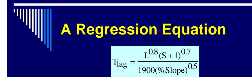
where :  $T_{lag}$  = lag time in hours L = Length of the longest drainage path in feet S = (1000/CN) - 10 (CN=curve number) %Slope = The average watershed slope in %
