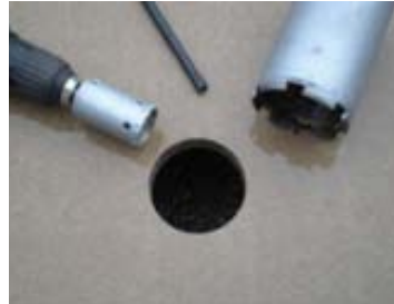
Top: Left and Right: Installation of J clip bracketing hardware. Bottom Left and Right: typical conventional coring and cutting tools used with ARCIS panels.
