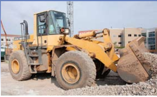
This Komatsu WA380 wheel loader is used for a variety of tasks, such as cleaning up rock and carrying pipe.
