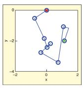
Figure 1. The locations of a Brownian particle on the x-y plane, observed at a fixed interval of time, and on a preestablished length scale. The particle starts at the origin (red circle), and ends at the tenth observation (green circle).
