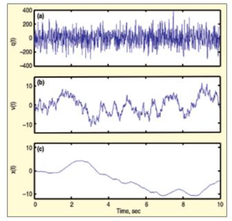
Figure 4. (a) Sample excitation from a band-limited random source with two-sided spectral density,  $S_{ww} = 1 \ lb^2/(rad/sec)$ , with frequency content in [-50,50) Hz; (b) velocity response of structure of Figure 2, with  $m = 1 \ lb-sec^2$ /in, and  $c = 1 \ lb-sec/in$ , to the input in Figure 4a. (c) displacement response of the structure of Figure 2, with  $m = 1 \ lb-sec^2/in$ , and  $c = 1 \ lb-sec/in$ , to the input in Figure 4a.
