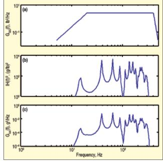
Figure 8. (a) Spectral density of a stationary, Gaussian force random process that is input to a structure; (b) modulus squared of the frequency response function of a single-input/single-output structure (FRF relates input force to response acceleration); (c) spectral density of the random acceleration structural response.
