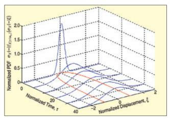
Figure 6. Six marginal PDFs of the displacement response of an SDOF structure developed by Uhlenbeck and Ornstein.^{12}
