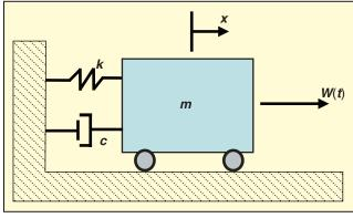
Figure 5. Single-degree-of-freedom (SDOF) structure with mass m stiffness k and damping c excited by input force W(t).
