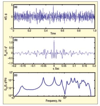
Figure 7. (a) Realization of a stationary random process; (b) estimated autocorrelation function of the source of the random signal in Figure 7a; (c) estimated spectral density function of the source of the random signal in Figure 7a.
