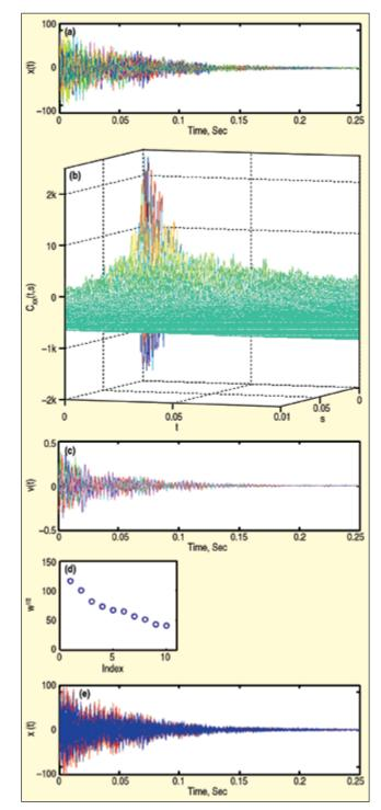
Figure 10. (a) Twenty realizations from a nonstationary random source; (b) estimated covariance of the random source of the signals in Figure 10a; (c) estimated shape functions of the KLE of the source of signals in Figure 10a; (d) estimated amplitudes of the KLE of the source of the signals in Figure 10a; (e) generated realizations (red) from the approximate source of the realizations in Figure 10a (blue), assuming that U is jointly Gaussian.
