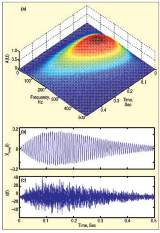
Figure 9. (a) Surface plot to the amplitude/frequency term  $A_{kj}$  in a stochastic representation of a nonstationary random process; (b) one component of a nonstationary random process realization with  $A_{kj}$  from Figure 9a; (c) one realization from a nonstationary random process with  $A_{kj}$  from Figure 9a.
