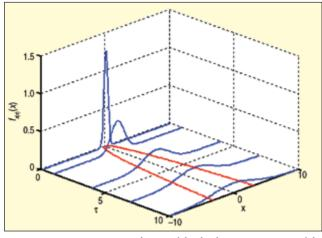
Figure 3. Five separate marginal PDFs of the displacement response of the system in Figure 2 at normalized times  $\tau = 2Dt = 0.1, 1, 4, 7, 10$ . (Blue, Eq. 2a, plotted above the  $\tau - x$  plane) Standard deviation of the response. (Red, Eq. 2b, plotted in the  $\tau - x$  plane).
