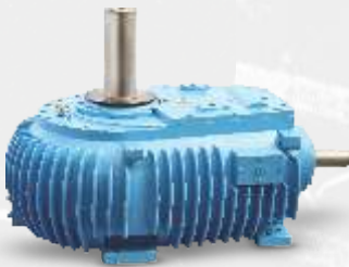
10. ELECON - ET SERIES SPIRAL BEVEL CUM HELICAL GEARBOX WITH VERTICALLY UPWARD OUTPUT SHAFT FOR COOLING TOWER APPLICATION. Ratio : 8.....16 Power : 14.....1000 kW Torque : 80 KNm
