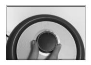
Adjust the Temperature Control Dial to the specified temperature.
