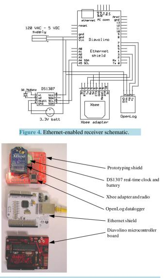
Figure 5. Ethernet-enabled receiver components.
