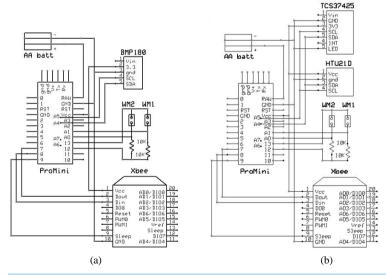
Figure 2. Schematics for (a) Field transmitter #1, and (b) Field transmitter #2.
