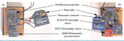
Figure 3. Components of (a) Field transmitter #1 and (b) Field transmitter #2.
