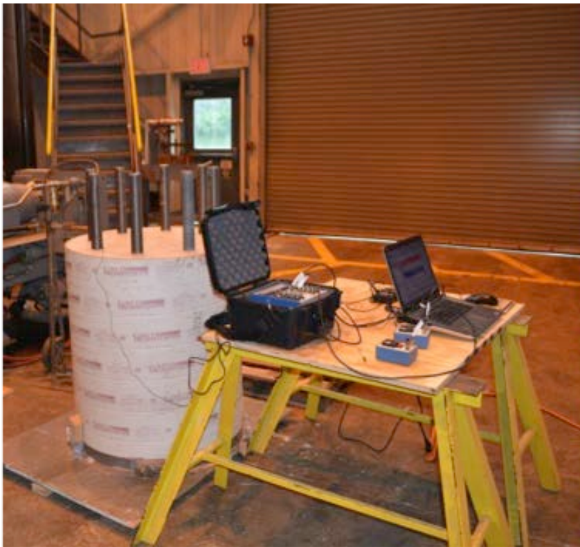
FIGURE 13 Test set-up for embedded rods without base plate, washers and nuts.
