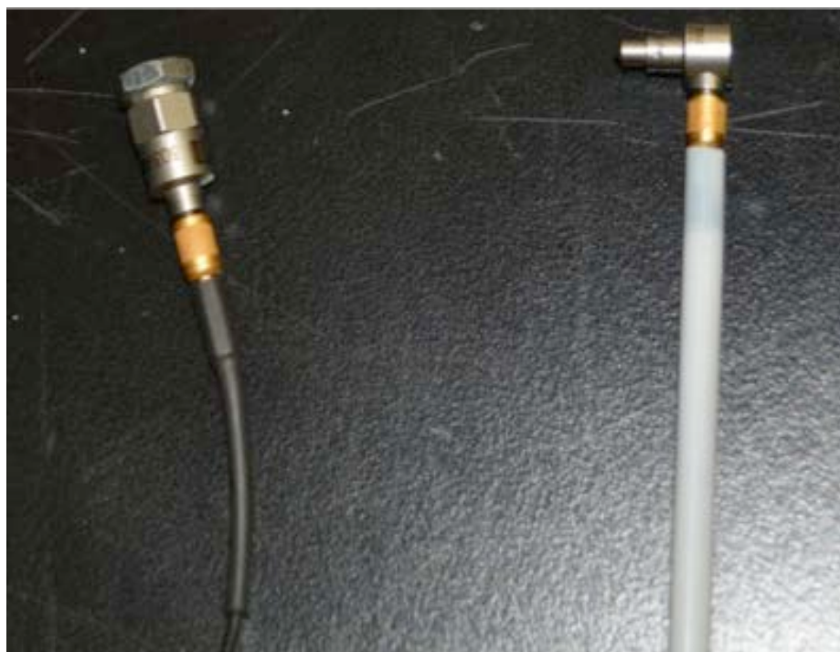
FIGURE 8 PCB piezoelectric accelerometer (left) and instrumented hammer (right).
