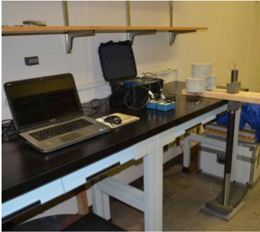
FIGURE 12 Test set-up for a single isolated anchor rod.
