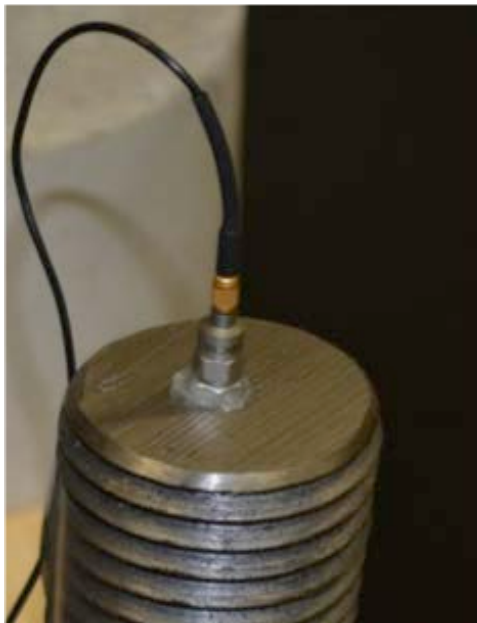
FIGURE 10 Accelerometer mounted on the top surface of a test rod with high vacuum grease coupling agent.
