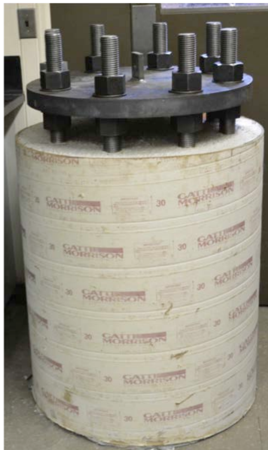
FIGURE 7 Photograph of the completed structure-foundation test specimen.
