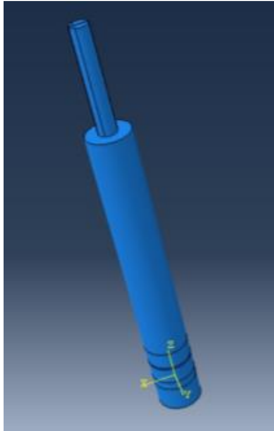
FIGURE 29 Finite element model of the embedded rod assembly.
