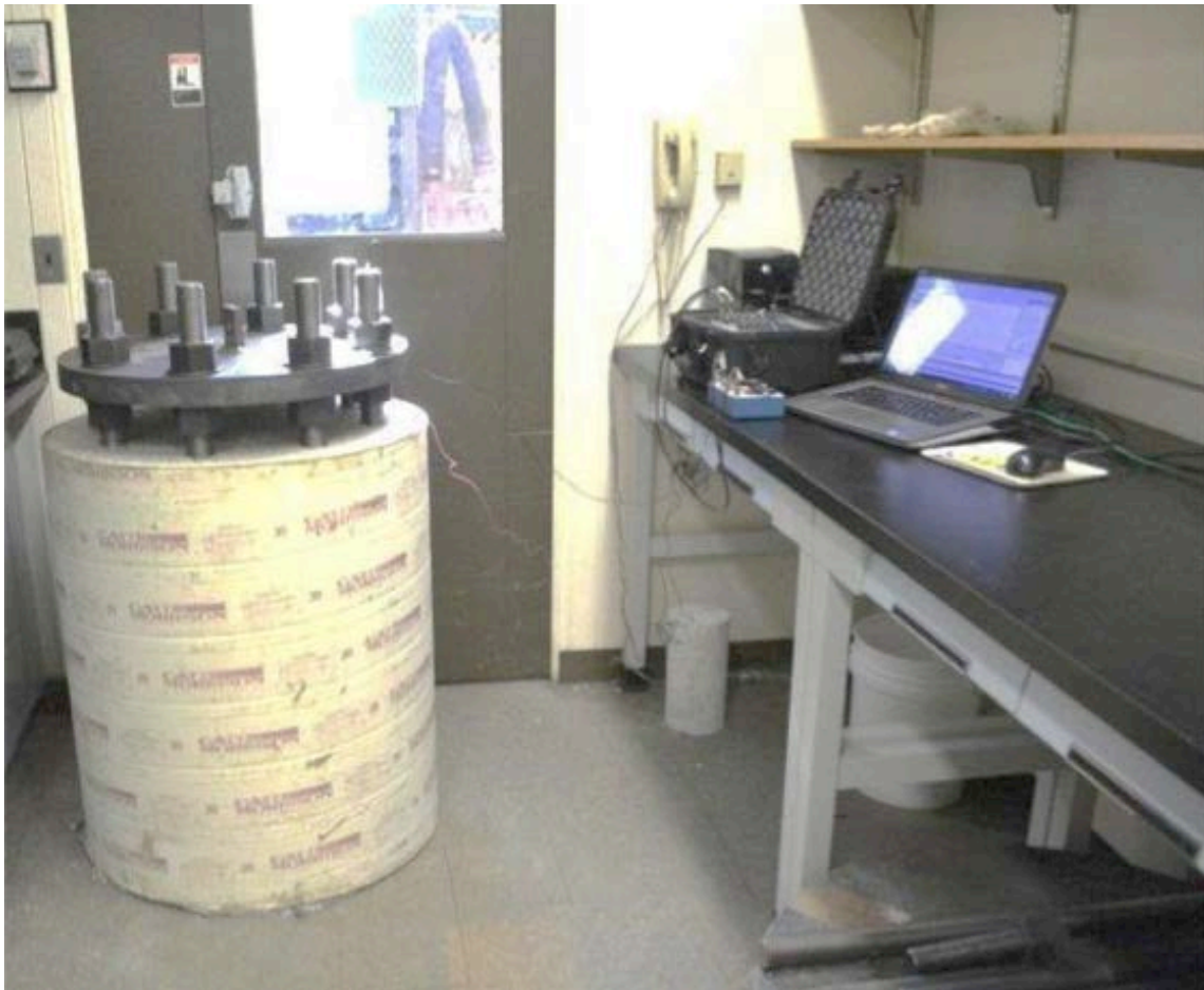
FIGURE 16 Baseline testing of the completed structure-foundation anchorage assembly.
