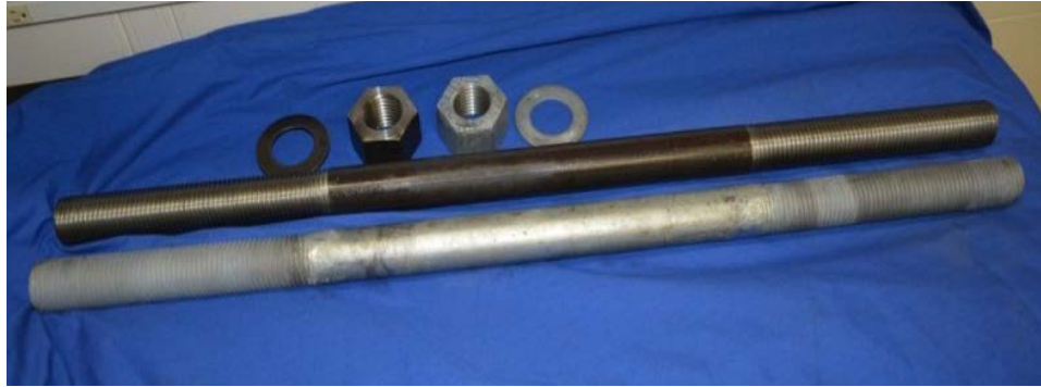
FIGURE 6 Photograph of anchor rods, nuts and washers.
