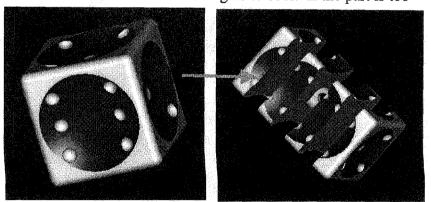
Figure 2 Example of Thick Part Decomposition
