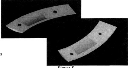
Figure 5 Interlocking Features Created Using the Ejector Pins
