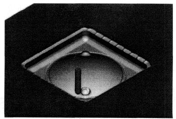
Figure 6 Simulation of NC Machining of Mold Cavities
