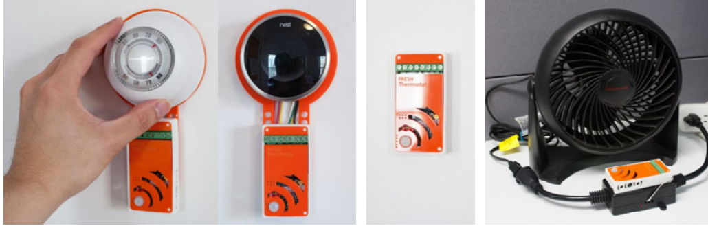
Figure 10. Different setups for the FRESH Thermostat: interfaced with an analog and smart thermostat to monitor their relay states for controlled experiments (Left), interfaced directly to control the central HVAC (Middle), and interfaced with a plug-controlled fan (Right).
