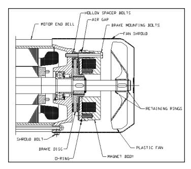
Figure 5-8a. ABM Motor Brake
