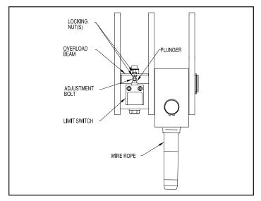
Figure 7-3b. Over-Capacity Limit Switch ("D" Frame)
