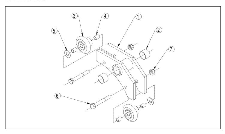
Figure 9-7b. Rope Guide Assembly (S4 & S2 Reeved)
