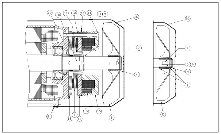
Figure 9-9b. Outdoor Service Hoist Motor Brake (ABM Motor)
