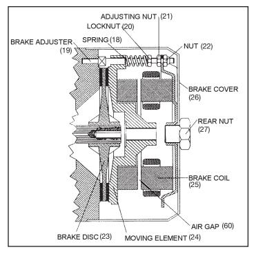
Figure 5-8b. MGM Motor Brake
