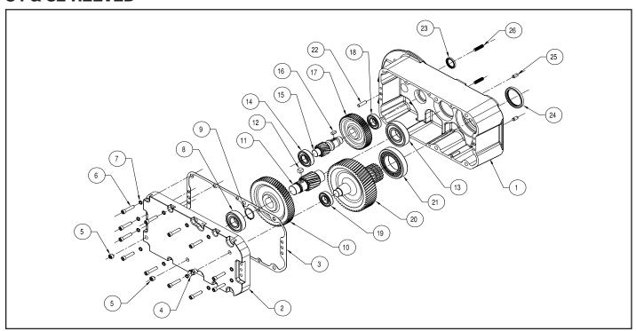
Figure 9-2. Hoist Gearing
