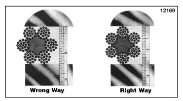
Figure 5-4. Correct Method of Measuring Rope
