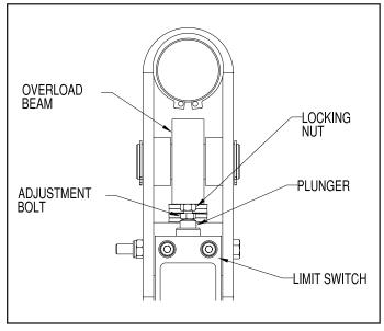
Figure 7-3a. Over-Capacity Limit Switch ("B" & "C" Frame)
