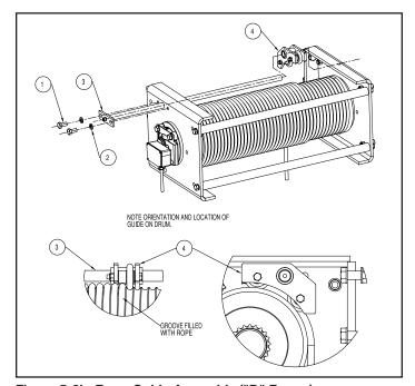
Figure 5-3b. Rope Guide Assembly ("D" Frame)
