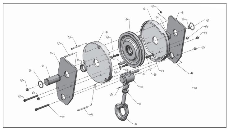
Figure 9-4b. Lower Block Assembly (S2 Reeved)
