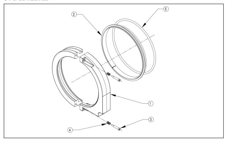
Figure 9-7a. Rope Guide Assembly ("B" & "C" Frame) (S4 & S2 Reeved)
