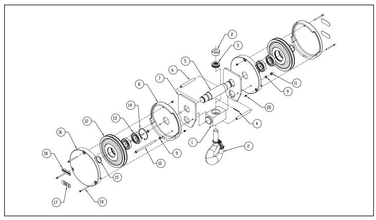
Figure 9-4a. Lower Block Assembly (S4 Reeved)
