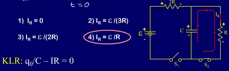
Recall q is charge on capacitor after charging:  $q_0 = \varepsilon C$  (since charged w/ switch 2 open!)  $\varepsilon - IR = 0 \implies I = \varepsilon /R$
