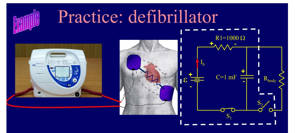
A 500 V battery is used to charge the 1 mF capacitor for 2 seconds. How much energy is stored in the capacitor?
