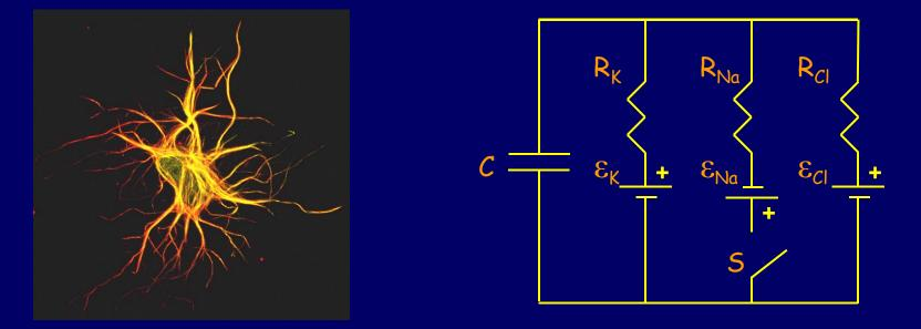
With resistance in the circuits, capacitors do not charge and discharge instantaneously – it takes time (even if only fractions of a second).
