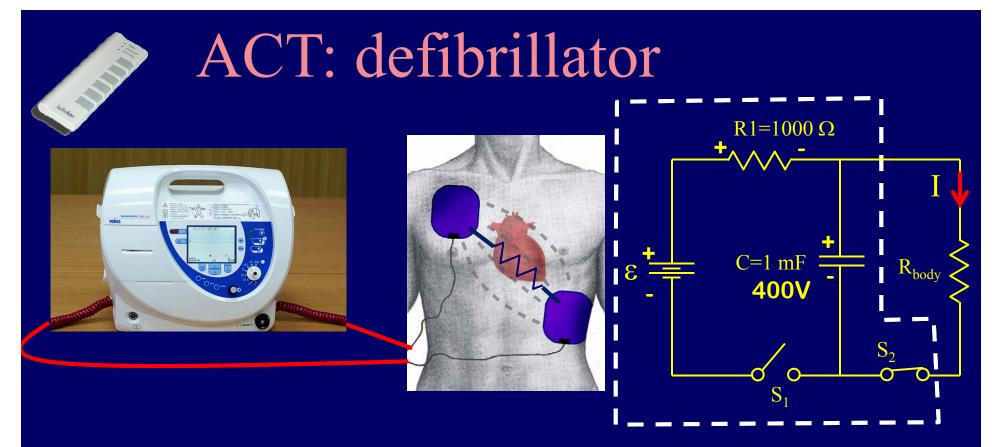
After charging for 2 seconds,  $S_1$  is opened; What is the current through the patient right after  $S_2$  is closed if  $R_{body}$ =100  $\Omega$ ? (A) 0 A (B) 4 A (C) 0.25 A
