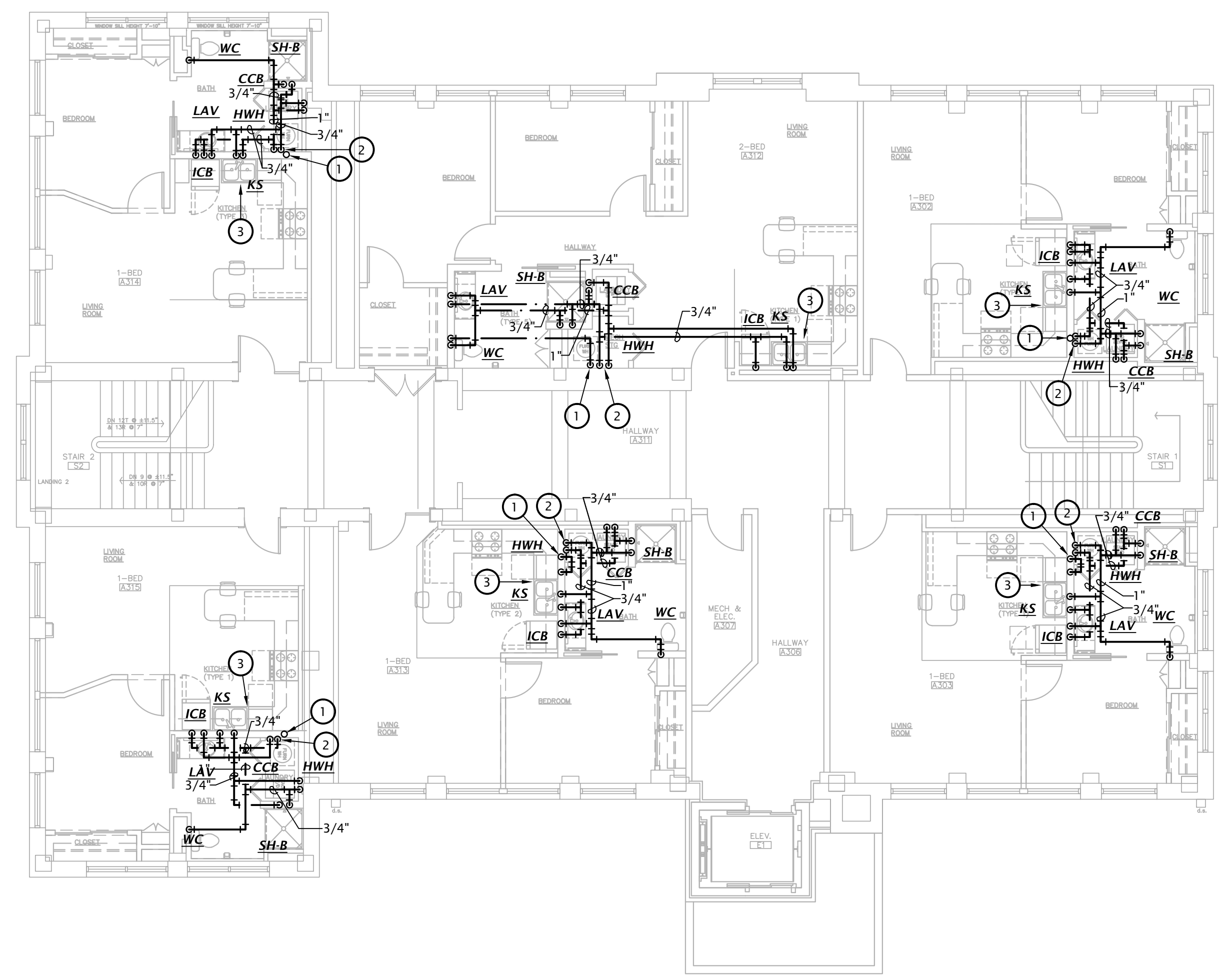
1 BUILDING A FIRST FLOOR DOMESTIC WATER PLAN 1/8" = 1'-0"
