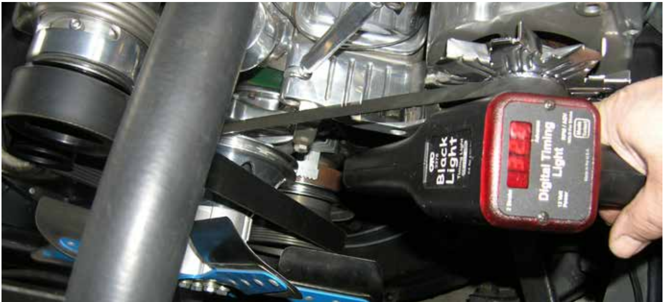
A dial-back timing light is a good way to check the advance curve if you do not have access to a distributor test stand.
