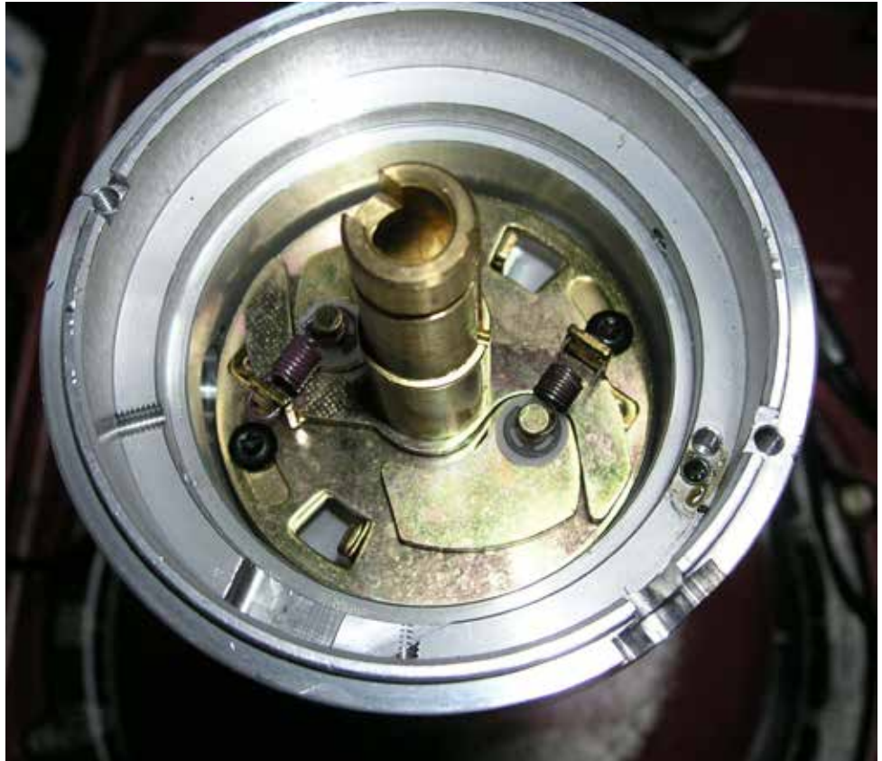
This is the advance system that is in the newer Mallory, Accel, and MOPAR Performance distributors.
