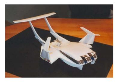
Figure 6: The HW-80 showing the blended/lifting body/hull and folding wings
