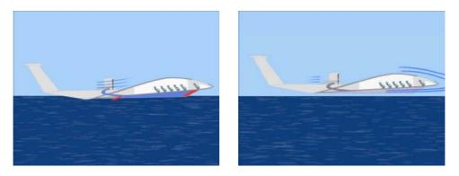
Figure 4: Illustration of retractable SES air cushion as craft makes transition from 'hovercraft'/step-taxi mode (left) to WIG mode (right).
