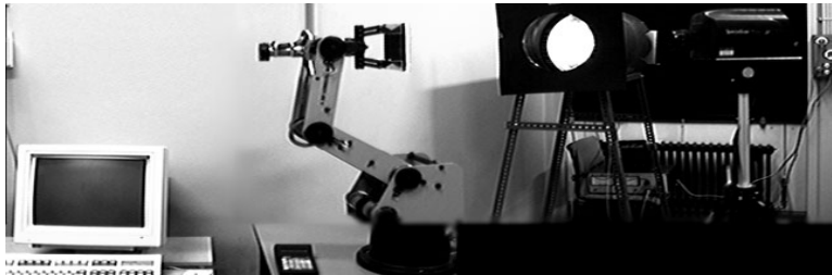
Fig. 2. Measurement setup. The equipment consists of a personal computer with a 24-bit R/G/B frame grabber, a robot arm to orient the texture samples, a halogen bulb with a Fresnel lens which produces a parallel beam, a photometer and a 3-CCD color video camera (not shown).
