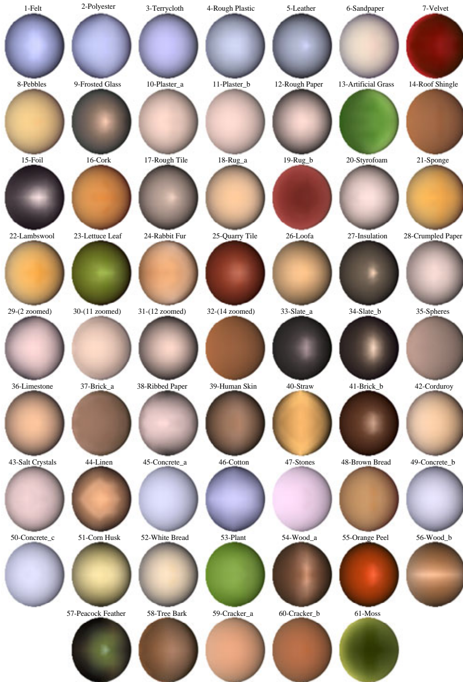
Fig. 14. Spheres rendered using the BRDF measurements obtained from camera position 1 (illumination at 22.5^\circ to the right). Interpolation was used to obtain radiance values between the measured points.
