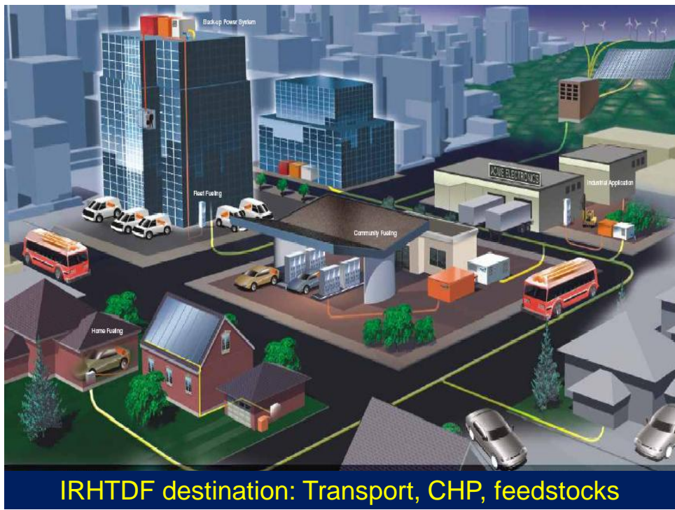
Figure 4. At IRHTDF destination, high-purity GH2 is distributed for transportation and stationary CHP fuel and for industrial feedstocks, via extant and / or new underground pipelines immune to HE, HCC.
