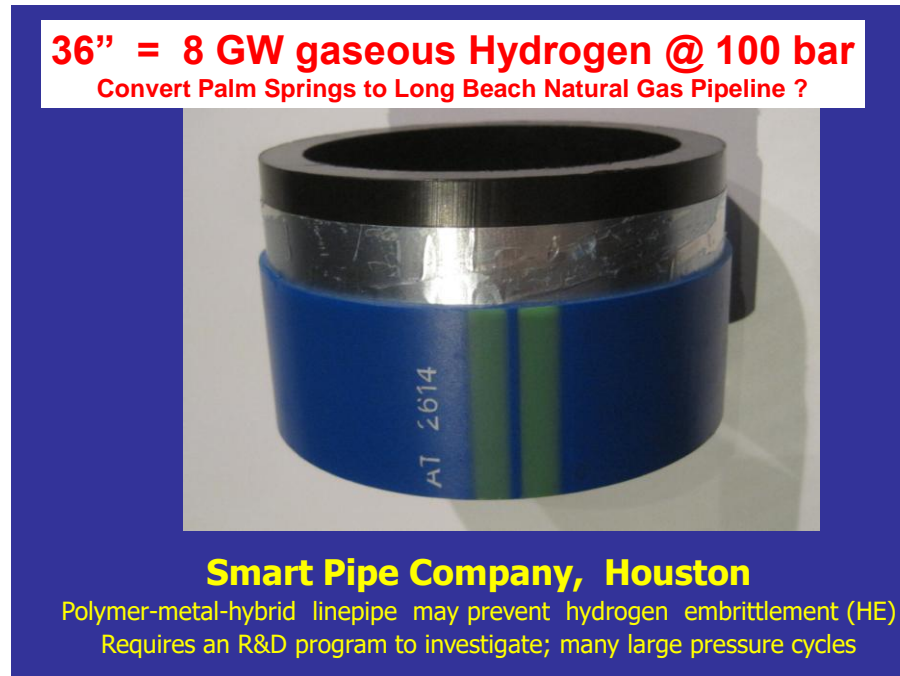
Figure 5. A Smart Pipe Company concept sample, circa 2005, but not intended for, nor tested for, high-purity GH 2 in VER service. HDPE core. A thin layer of Cu or Al in pipe wall is the H 2 permeation barrier: might be a spiral-wrapped foil with laser-welded seams or metal spray deposition. FRP overwrap (not shown here) accepts maximum allowed operating pressure (MAOP).
