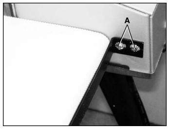
3. Using the supplied hex wrench, remove both conveyor table mounting bolts(B) on the open side of the sander. **SEE FIG 15.**
