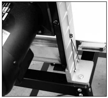
2. Using two wood blocks of **IDENTICAL** height, place one at Measurement A and one at Measurement B. **SEE FIG. 10.**
