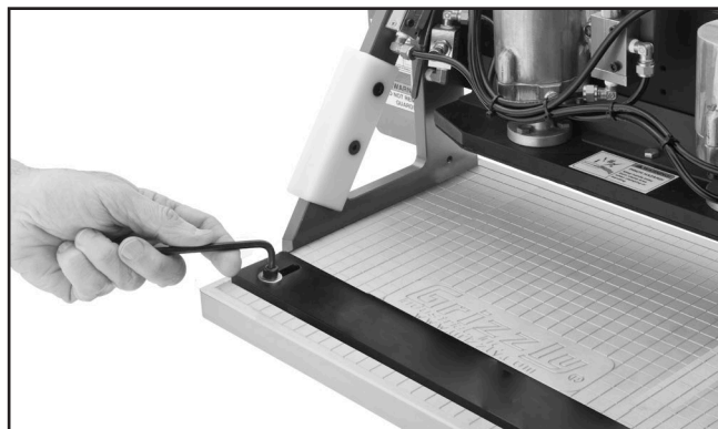
Figure 11. Securing the rear fence using M6-1 x 16 cap screw (1 of 2).
