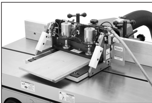
Figure 18. Shaping jig prepared for use with shaper OFF .
