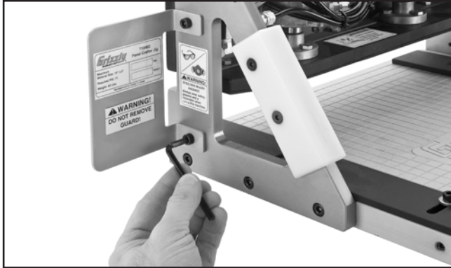
Figure 4. Attaching guard to jig.
