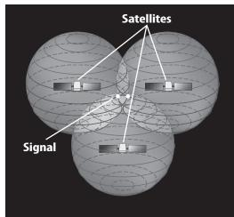
The distance between each satellite is calculated. The location of the GPS receiver has to be somewhere within the area where the spheres intersect. By using three satellites, the location of the receiver can be calculated to be one of two points.
