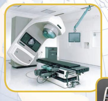
nomosSTAT<sup>™</sup> serial tomotherapy technology delivers pencil beams from a continuous 340-degree arc around the patient, creating a highly conformal dose distribution. Treatments delivered with nomosSTAT provide better critical structure avoidance than other IMRT techniques without compromising dose to the target. These capabilities can be added to any linear accelerator while maintaining the ability to deliver conventional treatments.
