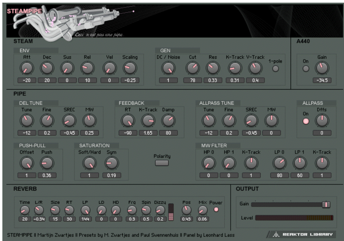
Fig. 1.25 Steam Pipe user interface
