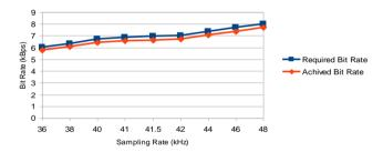
Figure 11: Bit rate vs sampling rate in audio throughput of tx & rx
