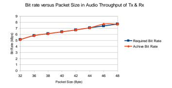
Figure 12: Bit rate vs packet size in audio throughput of tx & rx
