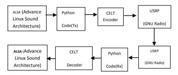
Figure2: Basic Architecture of CELT implemented in Linux platform
