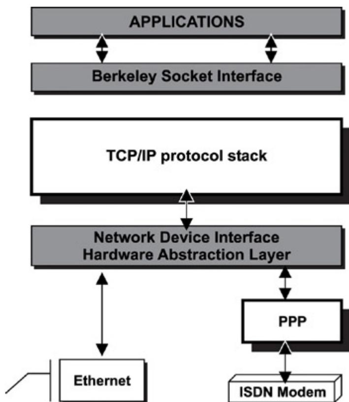
Figure 9.2: TCP/IP protocol stack component.
