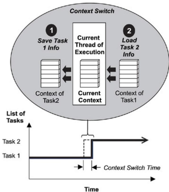
Figure 4.3: Multitasking using a context switch.
