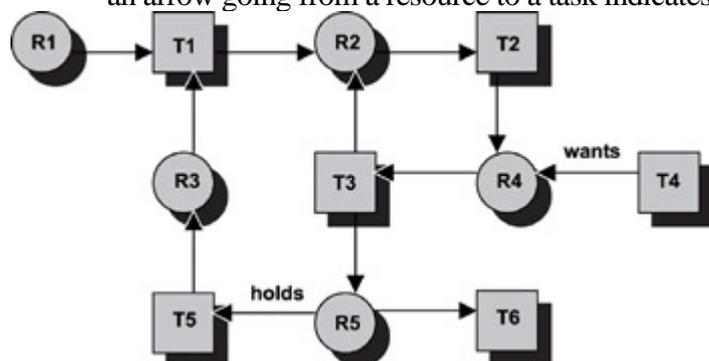
Figure 16.3: Current state of resource allocations and requests.
