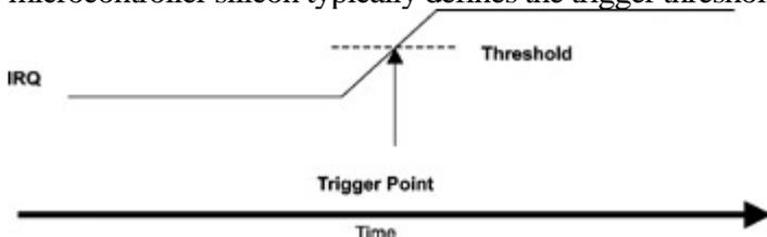
Figure 10.12: Level triggering.
