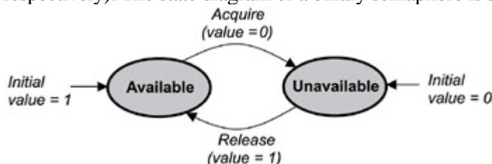
Figure 6.2: The state diagram of a binary semaphore.
