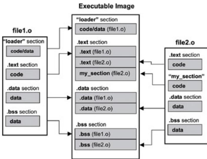
Figure 2.6: Combining input sections into an executable image.
