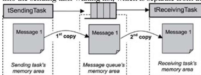
Figure 7.3: Message copying and memory use for sending and receiving messages.
