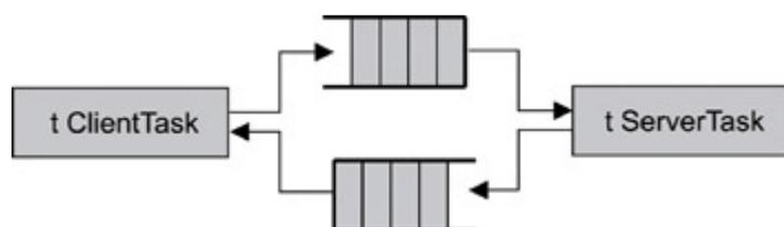
Figure 7.8: Interlocked, two-way data communication.
