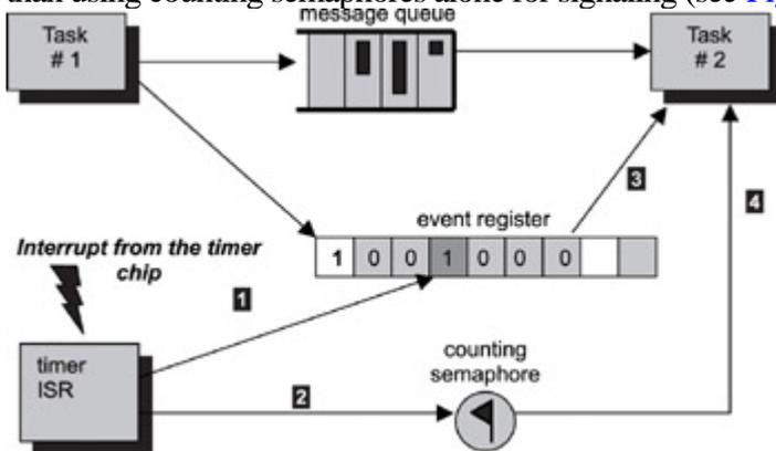
Figure 15.19: Task with multiple input communication channels.
