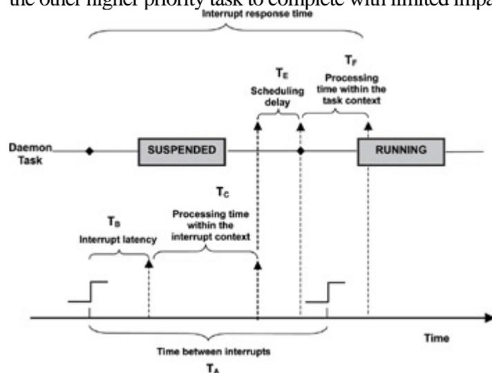
Figure 10.10: Interrupt processing in two contexts.
