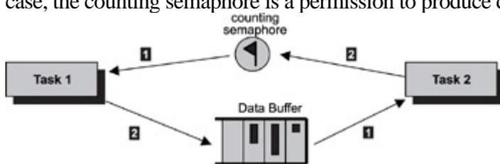
Figure 15.17: Using counting semaphores for flow control.
