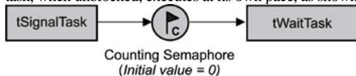
Figure 6.7: Credit-tracking synchronization between two tasks.
