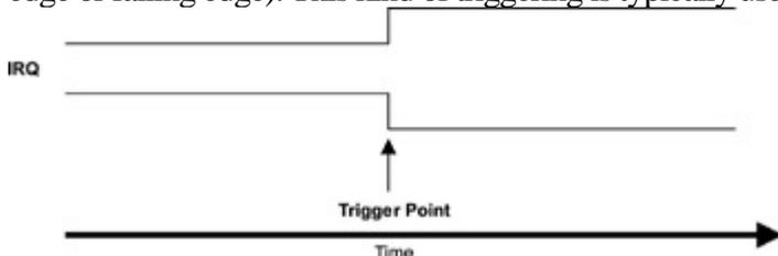
Figure 10.11: Edge triggering on either rising or falling edge.
