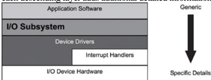
Figure 12.1: I/O subsystem and the layered model.
