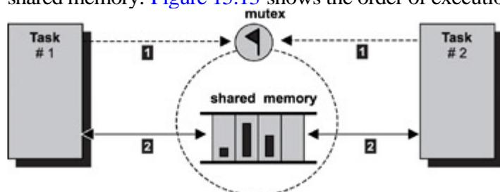
Figure 15.13: Task-to-task resource synchronization-shared memory guarded by mutex.
