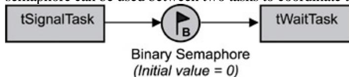
Figure 6.5: Wait-and-signal synchronization between two tasks.
