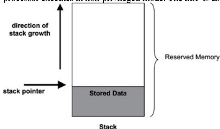
Figure 10.3: Store processor state information onto stack.
