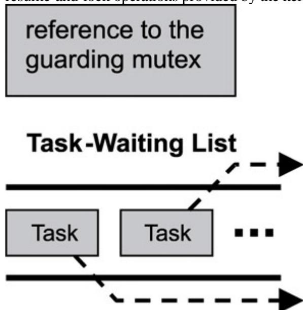
Figure 8.14: Condition variable control block.
