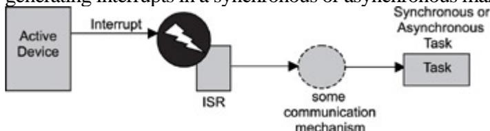
Figure 14.5: General communication mechanisms for active I/O devices.
