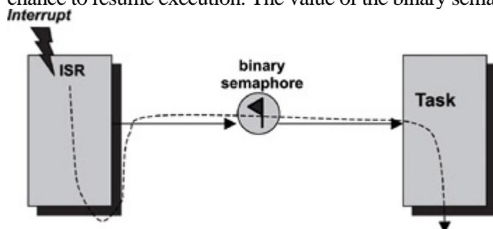
Figure 15.7: ISR-to-task synchronization using binary semaphores.
