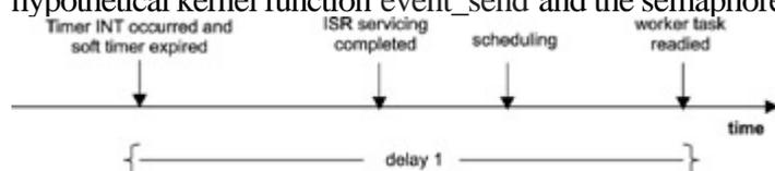
Figure 11.6: Level 1 delays-timer event notification delay.
