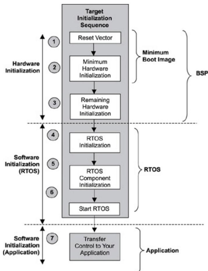
Figure 3.7: The software initialization process.
