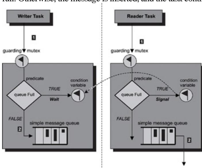
Figure 15.20: Using condition variables for task synchronization.
