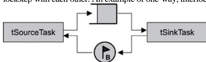
Figure 7.7: Interlocked, one-way data communication.
