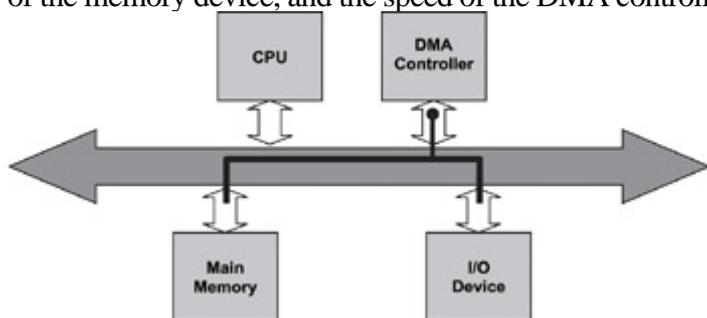
Figure 12.4: DMA I/O.
