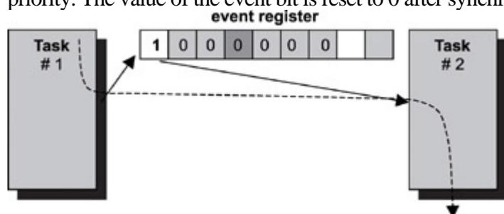
Figure 15.8: Task-to-task synchronization using event registers.
