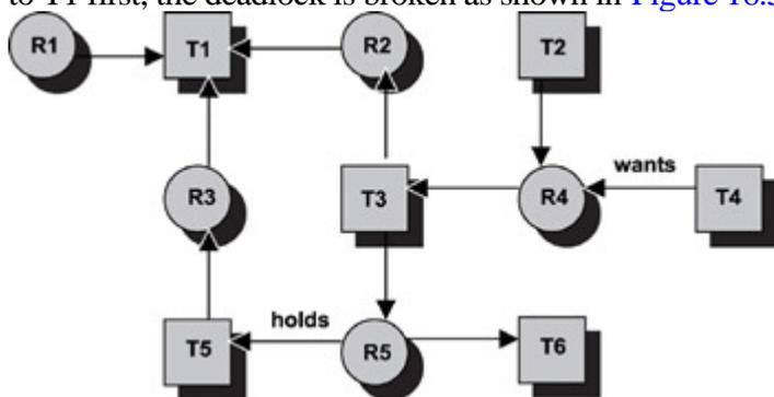
Figure 16.5: Deadlock eliminated by proper resource reassignment.
