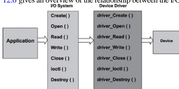
Figure 12.6: I/O function mapping.
