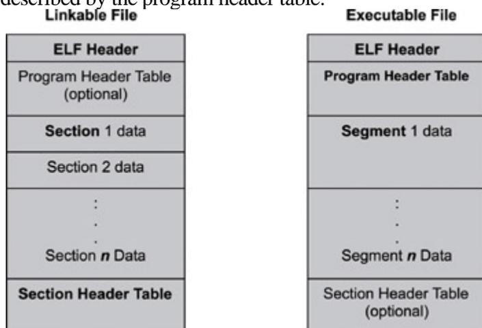
Figure 2.4: Executable and linking format.
