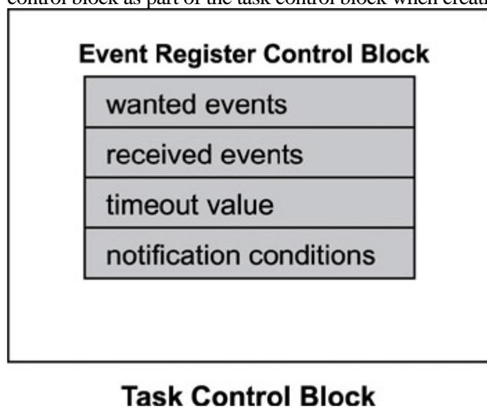
Figure 8.8: Event register control block.
