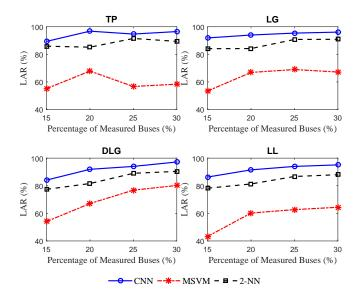
Fig. 4: The LAR of the CNN, MSVM, NN on the four types of faults in terms of different percentage of measured buses
