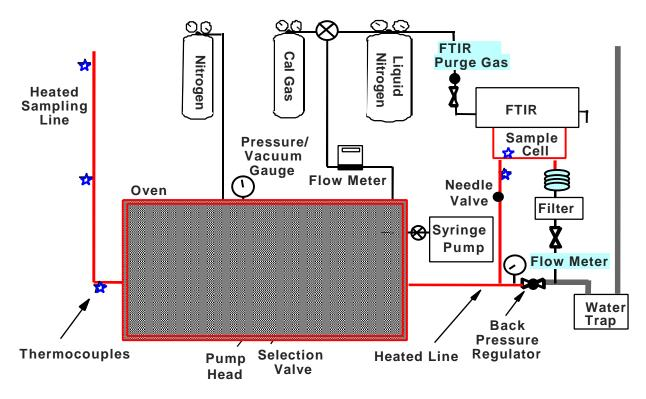
FIGURE 2. FTIR SAMPLING SYSTEM
