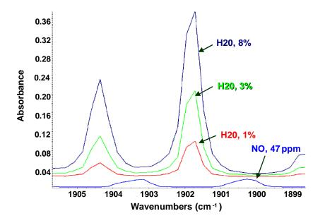
FIGURE 9. FTIR CALIBRATION SPECTRA OF H<sub>2</sub>O AND NO—REGION SELECTED FOR NO ANALYSIS
