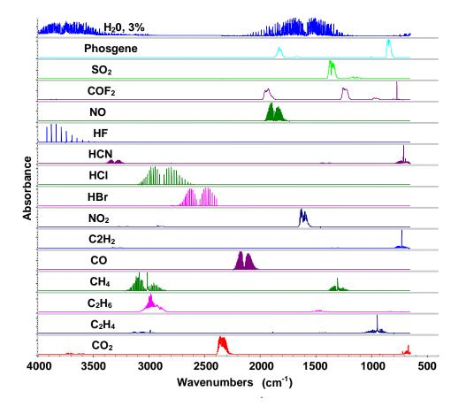
FIGURE 6. FTIR CALIBRATION SPECTRA OF 16 GASES AT 170?C-FULL-SCALE
