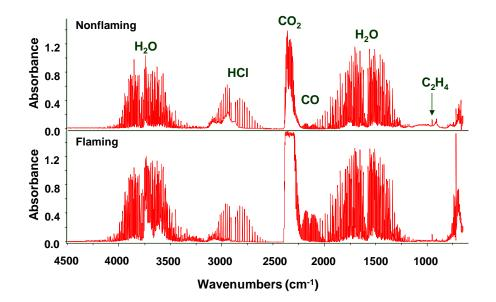
FIGURE 14. FTIR SPECTRA OF NONFLAMING AND FLAMING MIXED PLASTIC SPECIMENS AT 171 SECONDS
