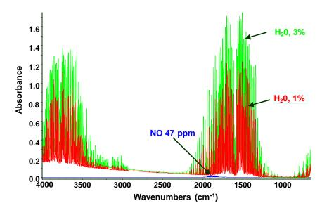
FIGURE 8. FTIR CALIBRATION SPECTRA OF H<sub>2</sub>O AND NO
