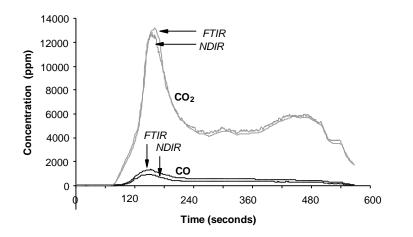
FIGURE 18. COMPARISON OF FTIR AND NDIR FLAMING PROFILES
