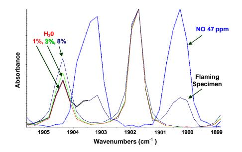
FIGURE 11. FTIR CALIBRATION SPECTRA OF H<sub>2</sub>O, NO, AND FLAMING SPECIMEN SPECTRUM—FULL SCALE
