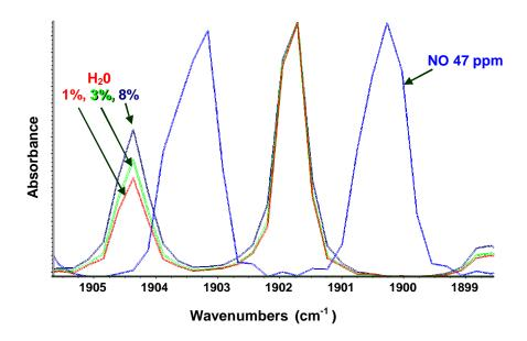
FIGURE 10. FTIR CALIBRATION SPECTRA OF H<sub>2</sub>O AND NO-FULL SCALE
