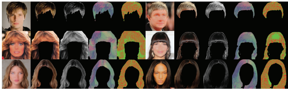
Fig. 3. Examples of our training data. For each set of images from left to right, we show input image; segmented hair; gray image; orientation map; and edge activation map
