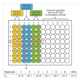
Figure 24. Plate setup for standard curve generation. When calculating the average threshold cycle  $\{C_t\}$  value, the highest and lowest values obtained from replicate reactions can be discarded.
