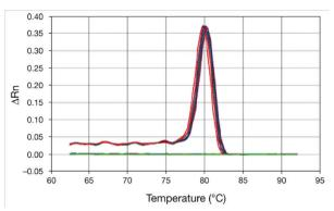
Figure 31. Amplification plots showing effects of poorly stored primers (shown by the melt curve and background fluorescence)
