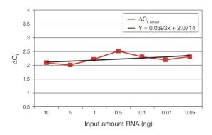
Figure 26. Relative efficiency plot. The  $\Delta C_1$  ranges from 2.0 to 2.5. When plotted against dilution or input amount of RNA, a slope is obtained. While a perfectly flat line (slope = 0) indicates identical efficiency across all input concentrations, a slope of <0.1 is generally considered acceptable when employing the  $\Delta\Delta C$ , method.
