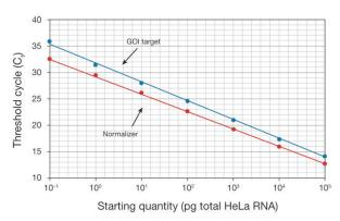
Figure 27. Efficiency values are obtained from standard curves to adjust the normalizer and gene-of-interest  $\mathbf{C}_t$  values. HeLa RNA was diluted over 6 orders of magnitude, and real-time PCR was performed to generate standard curves for both the normalizer and gene of interest (GOI).
