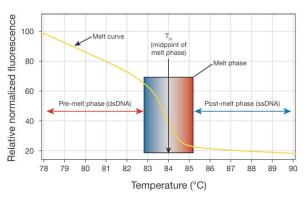
Figure 28. Characteristics of the melt curve profile for a PCR amplicon. Specific DNA sequences have characteristic melt-curve profiles. Mutations can be detected as either a shift in  $\boldsymbol{T}_m$  or a change in shape of the melt curve. In contrast to traditional melt curve analysis, HRM can distinguish between amplicons with just a single-nucleotide difference. This technique has opened the door to many new applications for dsDNA-binding dyes.
