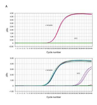
Figure 30. Amplification plots and melting profiles highlighting specific amplification (A) and primer-dimer effects (B). The primer-dimer can be identified in (B) by the signal produced by the NTC sample in the amplification plot, and additional peaks in the melting profile.
