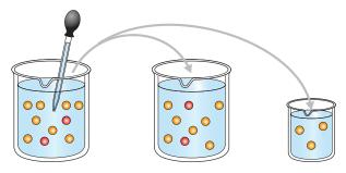
Figure 41. The Poisson principle assumes an appropriate volume of the total pool is sampled. Increasing the amount sampled from the total pool increases the ability to accurately determine the number of targets.
