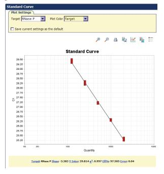
Figure 6. Amplification of RNase P DNA ranging from 1.25 x10³ to 2 x10⁴ copies. Real-time PCR of 2-fold serial dilutions of human RNase P DNA was performed using a FAM $^{\infty}$  dye-labeled TaqMan $^{\odot}$  Assay with TaqMan $^{\odot}$  Universal Master Mix II, under standard thermal cycling conditions on a ViiA $^{\infty}$ 7 Real-Time PCR System. (A) Amplification plot. (B) Standard curve showing copy number of template vs. threshold cycle (C<sub>i</sub>).
