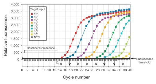
Figure 1. Relative fluorescence vs. cycle number. Amplification plots are created when the fluorescent signal from each sample is plotted against cycle number; therefore, amplification plots represent the accumulation of product over the duration of the real-time PCR experiment. The samples used to create the plots in this figure are a dilution series of the target DNA sequence.
