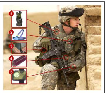
**Figure 10.** One version of integrated WPSM-IC including (1) fluid intake monitor, (2) vital signs detection system, (3) CPU hub, (4) temperature pill, and (5) actigraph (Buller et al. 2010).
