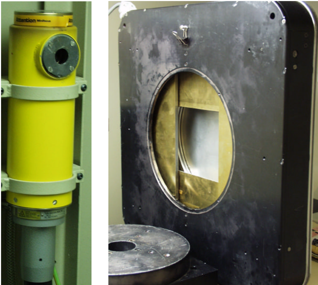
Figure 15. Photographs of a beam collimator mounted on the x-ray tube on the left and shutters mounted to the front of an image intensifier on the right.
