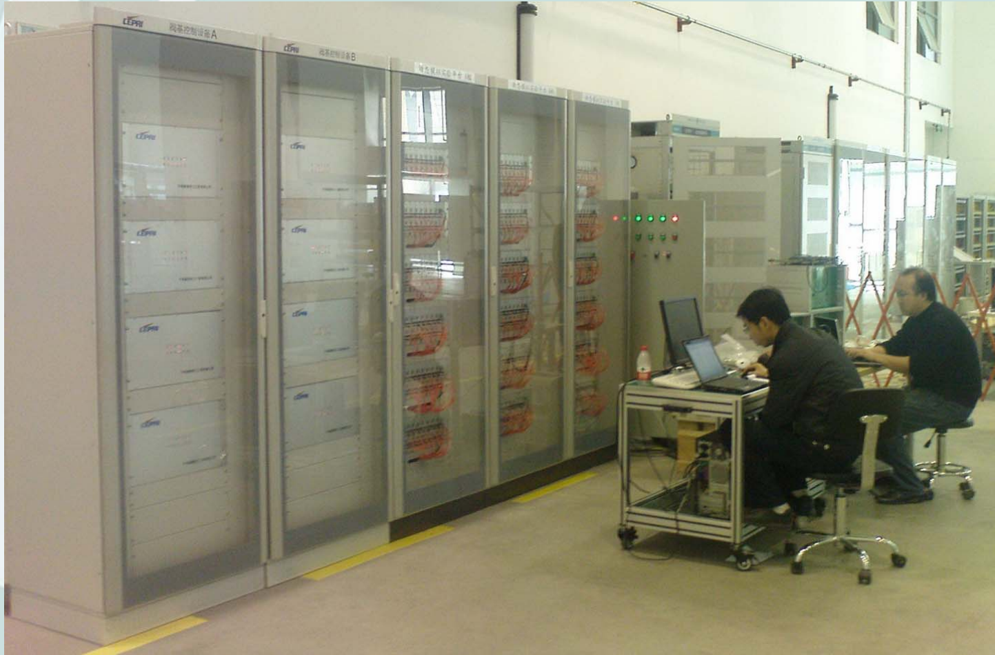
Picture of MMC-HVDC real time simulation platform
