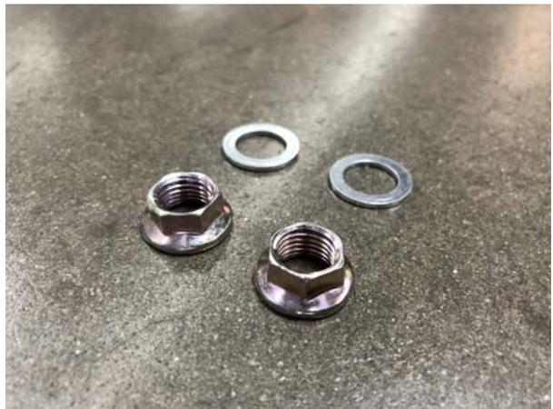
Insert a Jet nut onto each stainless steel caliper stud with a 12mm washer under each nut. Tighten the Jet nuts to **40 ft/lbs (54 n/m)** of torque, using a 1/2" socket.
