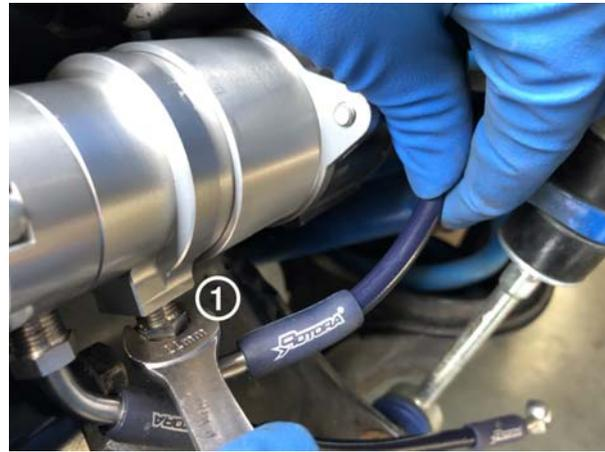
Determine the ② **LOWER LEFT-SIDE** stainless line's angle of rotation by presetting the Banjo fitting end to where the caliper inlet port location will be (as image shown below). You may temporarily mount the Rotor brake caliper onto the new bracket to determine the actual rotating angle. Once the position is confirmed, use an 11mm wrench to tighten the 135° swivel male-end fitting to **14 ft/lbs (19n/m)**.
