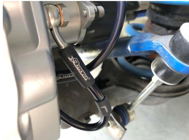
**NOTE:** Do not use a torque wrench, as over tightening the bolt can strip the aluminum threads, causing irreparable damage to the caliper.
