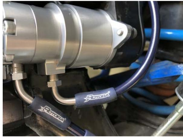
Determine the ① **UPPER** stainless line's angle of rotation by inserting temporarily the inboard end of the **UPPER** stainless steel brake line fitting through the existing hole of the locating bracket (as image shown). Once the position is confirmed, use an 11mm wrench to tighten the 90° swivel male-end fitting to **14 ft/lbs (19n/m)**.
