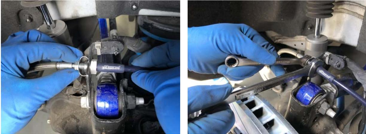
**NOTE:** Double check the **UPPER** stainless line clearance to ensure there is neither excessive binding tension, nor interference with any suspension components. Make necessary adjustment by re-clocking the 90° swivel male-end fitting to reposition.
