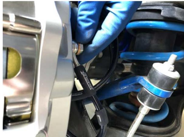
Be sure to orient the Banjo fitting (as image shown), with the **LOWER LEFT-SIDE** stainless line in a looped down position. Tighten the Banjo bolt using a 14mm wrench/socket and torque to approximately **14 ft/lbs (19n/m)**.
