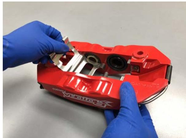
Insert one brake pad into position on one side of the caliper by setting the pad spring clip into tension. Then insert another brake pad onto the other side to set the spring clip into full tension. Ensure that the friction side of each brake pad is facing the brake disc.
