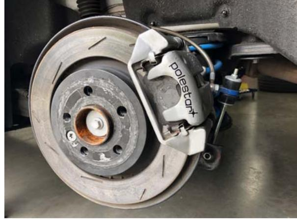
**⚠ WARNING:** Rotor recommends setting the vehicle to **SERVICE (MAINTENANCE) MODE** prior to the removal of the entire rear OEM brake system so that the Electronic Parking Brake (EPB) system can retract back to full release position. This procedure varies depending on the vehicle model and the diagnostic scanning software tool.
