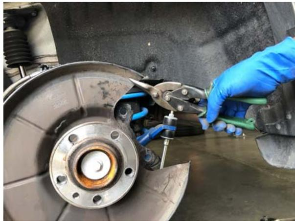
**NOTE:** Test fit the new 2-piece disc assembly. Rotate it to see if any portion of the dust shield would rub or comes in contact with it. You may strike the backing plate with a hammer in order to bend it back slightly to prevent interference. Use a file and smooth out the rough edges.
