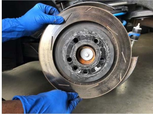
**NOTE:** It may be necessary to strike the brake disc on the outer edges with a rubber mallet if corrosion prevents the disc from coming off. If so, place a wheel lug in one of the holes first, to prevent the disc from falling when it comes loose.
