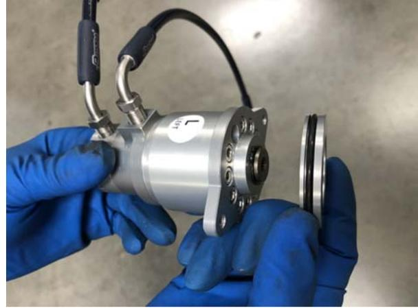
Using a T30 TORX bit, attach the original servomotor to the new EPBB module with the original 2 retaining screws.
