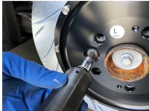
**NOTE:** Make sure the new disc is on the correct side of the vehicle. Reversing the discs will severely decrease the cooling capacity of the system. Refer to diagram on page 1 to determine direction.
