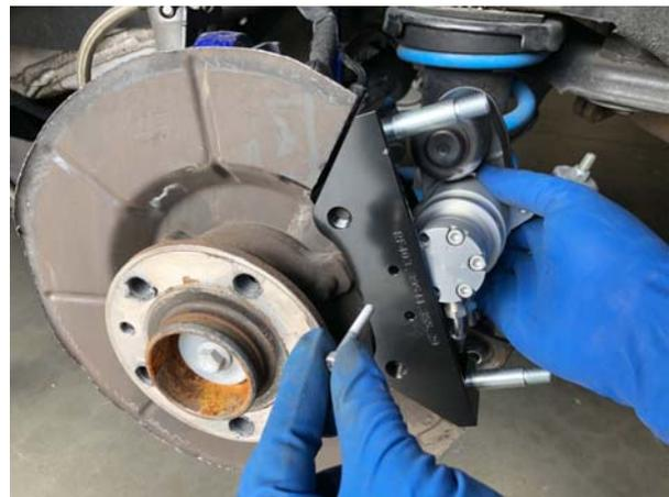
**NOTE:** Ensure that the orientation of the new **LEFT-SIDE EPBB-servomotor** assembly to the mounting bracket is positioned as image shown.
