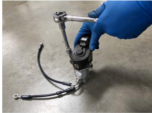
**NOTE:** Ensure that the orientation of the servomotor to the new **LEFT-SIDE EPBB** module is as image shown.
