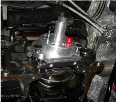
Torque for the bolts on the rear main seal flange is 11 ft-lbs.
