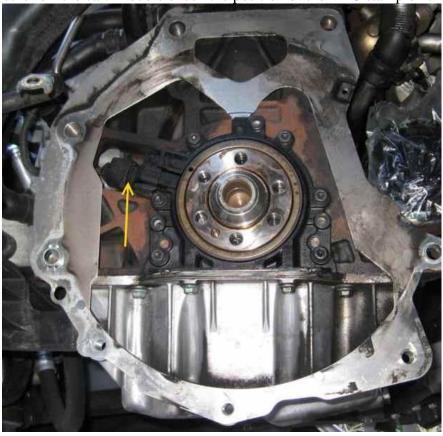
Pull the metal shim off. It will stick on the tab at the top and some transmission alignment dowels.
