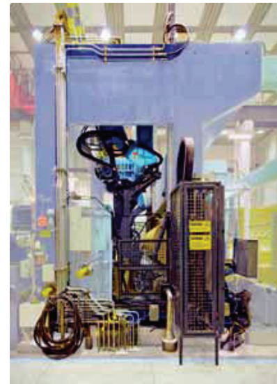
Figure 13. The rebuild improved safety by increasing the level of automation, moving the operator out of the machine area as much as possible.
