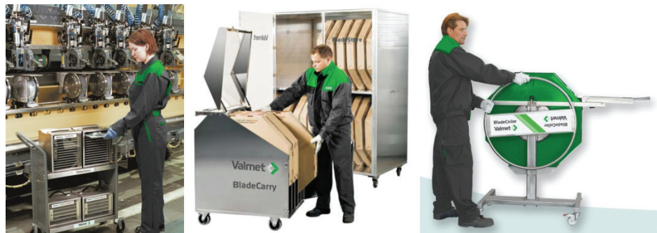
Figure 5. Storage and transportation methods such as SlitterCarry for slitter blades (left) and BladeStore and BladeCarry (middle) and BladeCoiler (right) for doctor blades improve the safety when operators handle and transport sharp consumables.
