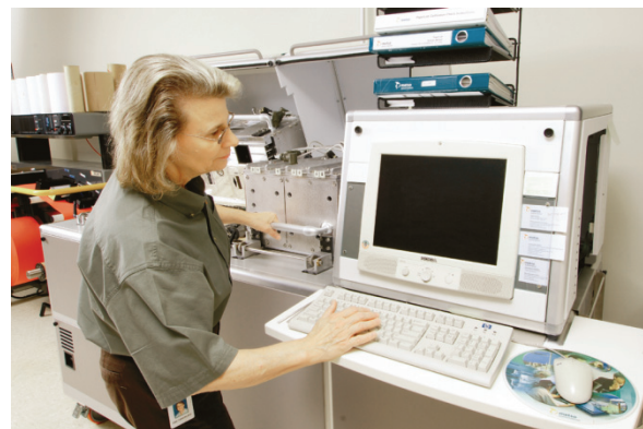
Figure 10. Valmet used a Tapio Analyzer (profiling) combined with state-of-the-art testing and analysis equipment acquired from the Beloit Rockton R&D Center.
