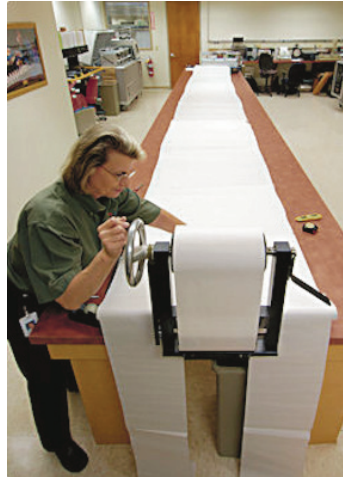
Figure 11. The mill's paper samples were processed by Valmet personnel, producing the frequency spectrum charts which they then analyzed further.
