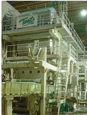
Figure 8. Tissue machine (left) reduced fires after Valmet yankee (right) received the new head covering, thereby increasing safety while reducing energy costs.
