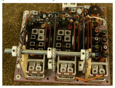
This is the same switch with the through screws and spacers removed. They are kept in order so that they may be replaced correctly.
