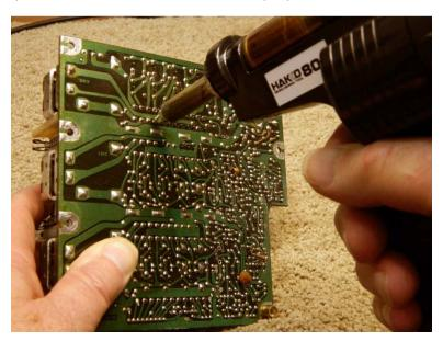
Using the Hakko 808, it is a simple matter to remove the solder around each wafer pin completely. When you have removed the solder from each pin, the wafer will fall out of the board.
