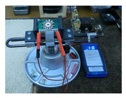
Each contact is checked for high resistance after cleaning. I am using here the Blue ESR meter which will measure quite low resistances. The reading here is .1 ohm. As you get closer to the other probe, the resistances will decrease as it is reading the resistance of the traces on the board. I also check physically for any looseness of the contact on the board. These contacts are originally held in place with rivets and they sometimes loosen.
