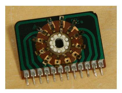
This is the first bandswitch wafer as removed from the RF board. You can see the buildup on the switch contacts and rotary contacts. This is not the worst I have seen by any means.
