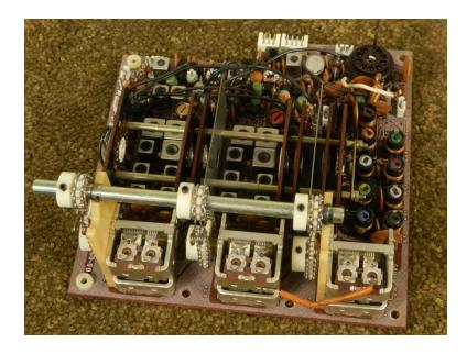
This is the RF board assembly as removed from the radio. It has only been cleaned by the use of compressed air to remove the loose dirt and dust.
