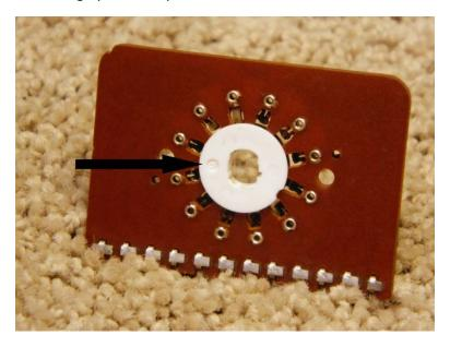
The rotary section of the switch must be properly aligned prior to installation so that each section will align properly with the switch shaft during reassembly. On the backside of the wafer are some marks that will be used for alignment. VERY IMPORTANT! Rotate the white collar of the switch so that the small recessed dot is at the nine o'clock position. When reassembling the switch, these will represent the 30 meter position on the bandswitch dial.
