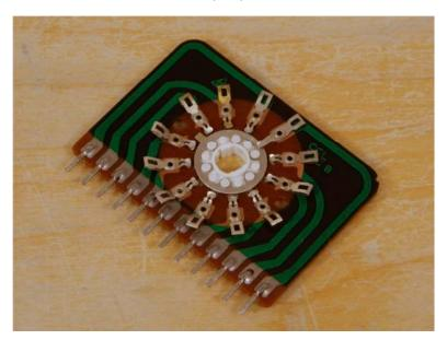
This is the same wafer after polishing to remove the tarnish on the contacts. I am now using a product made for polishing silver. It is called Wright's Silver Cream and works quite well. I use a discarded **soft** toothbrush to accomplish the cleaning/polishing and then rinse with tap water. The final rinse of the wafer is done with distilled water. The wafer is then carefully dried and blown out with canned air.
