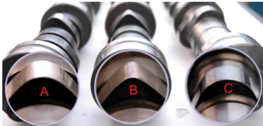
Figure 6. There are three camshafts for the 3208. Left to right, we have (A) flat tappet turbo; (B) non-turbo flat tappet; and (C) roller lifter turbo.
