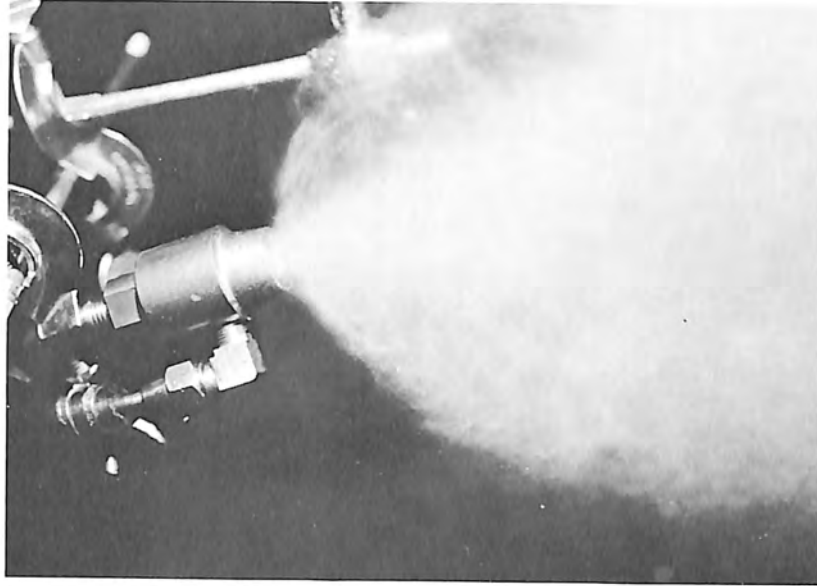
Figure 17. "Sonicore" No. 188 nozzle with air pressure = 60 psi (4.2 kg/cm 2 ), water pressure = 10 psi (0.7 kg/cm 2 ). Photo P801D-74385 NA
