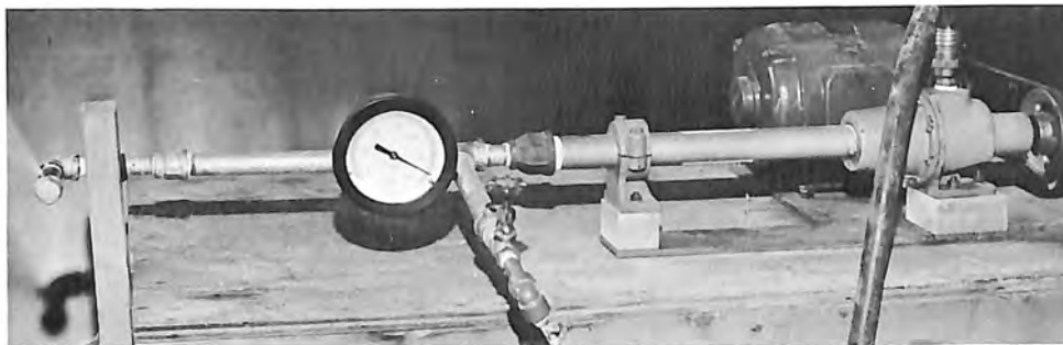
Figure 2. Equipment for injection through liquid nozzles. Photo P801D-74366 NA
