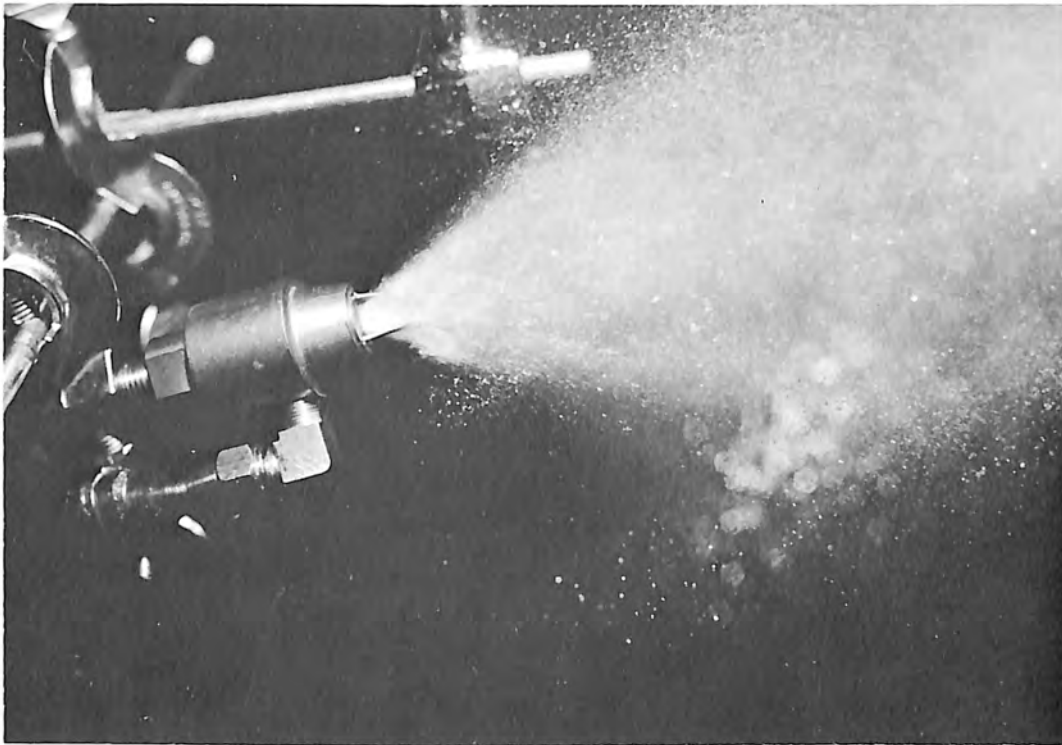
Figure 16. "Sonicore" No. 188 nozzle with air pressure = 10 psi ( 0.7 \text{ kg/cm}^2 ) water pressure = 60 psi ( 4.2 \text{ kg/cm}^2 ). Photo P801D-74384 NA
