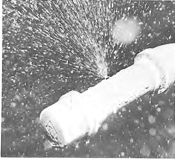
Figure 30. Self-impinging jets at 45 psi (3.2 kg/cm 2 ). Photo PX-D-71167NA
