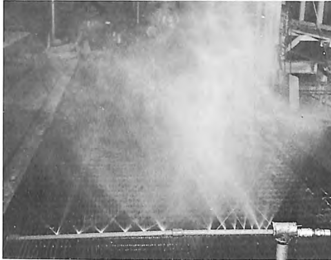
Figure 28. Series of self-impinging jet nozzles in operation. Photo P801D-74394NA
