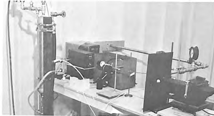
Figure 11. Spark-gap light source and optics for photographing airborne droplets. Photo P801D-74377 NA
