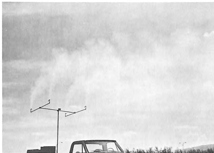
Figure 18. Ground-based spray rig using "Sonicore" nozzles for hygroscopic cloud seeding. Photo P801D-68982 NA
