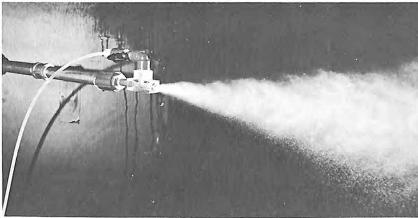
Figure 26. Prandtl-Meyer nozzle in operation. Photo P801D-74392NA
