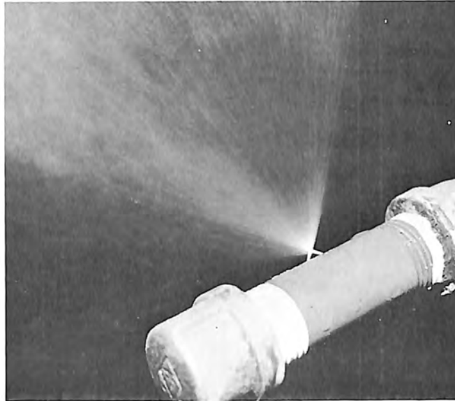
Figure 32. Self-impinging jets at 500 psi (35.2 kg/cm 2 ). Photo P801D-74398NA
