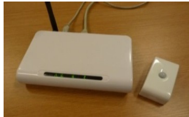
Fig. 4. A BuildAX logger/router/server (left) and multi-sensor environmental monitor.
