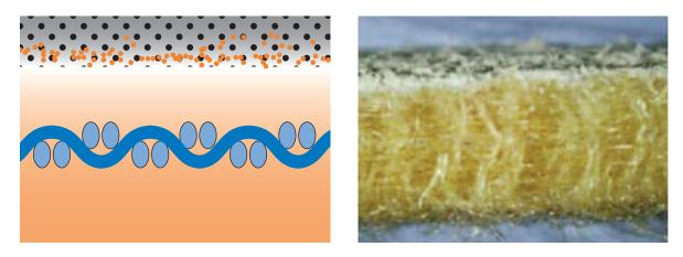
Figure 13 Needle felt filter schematic (Popovici, 2011)
