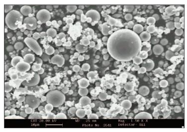
Figure 1 Typical fly ash photo (Barnes, 2010)
