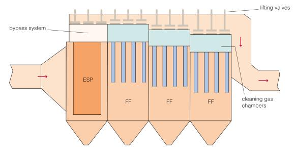
Figure 20 EFIC schematic (Zheng and others, 2011)
