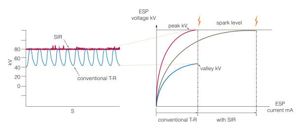
Figure 4 Ripple difference between SIR and conventional T-R (Ranstad and other, 2011)
