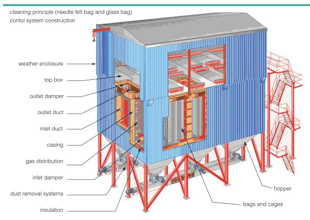
Figure 11 PJFF schematic (FLSmidth, 2012b)
