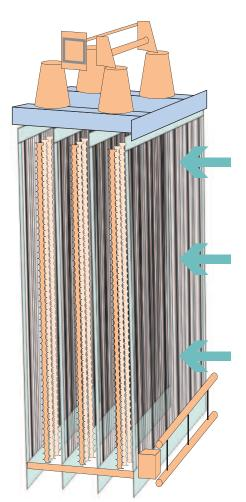
Figure 9 Cross flow ESP schematic (Back and Francis, 2006)
