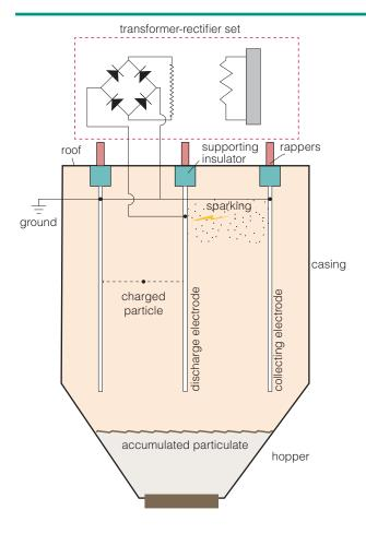
Figure 3 Dry ESP schematic (Majid and others, 2011; Grass and Zintl, 2008; Soud 1995)
