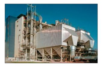
Figure 2 ESP photo (FLSmidth, 2012a)
