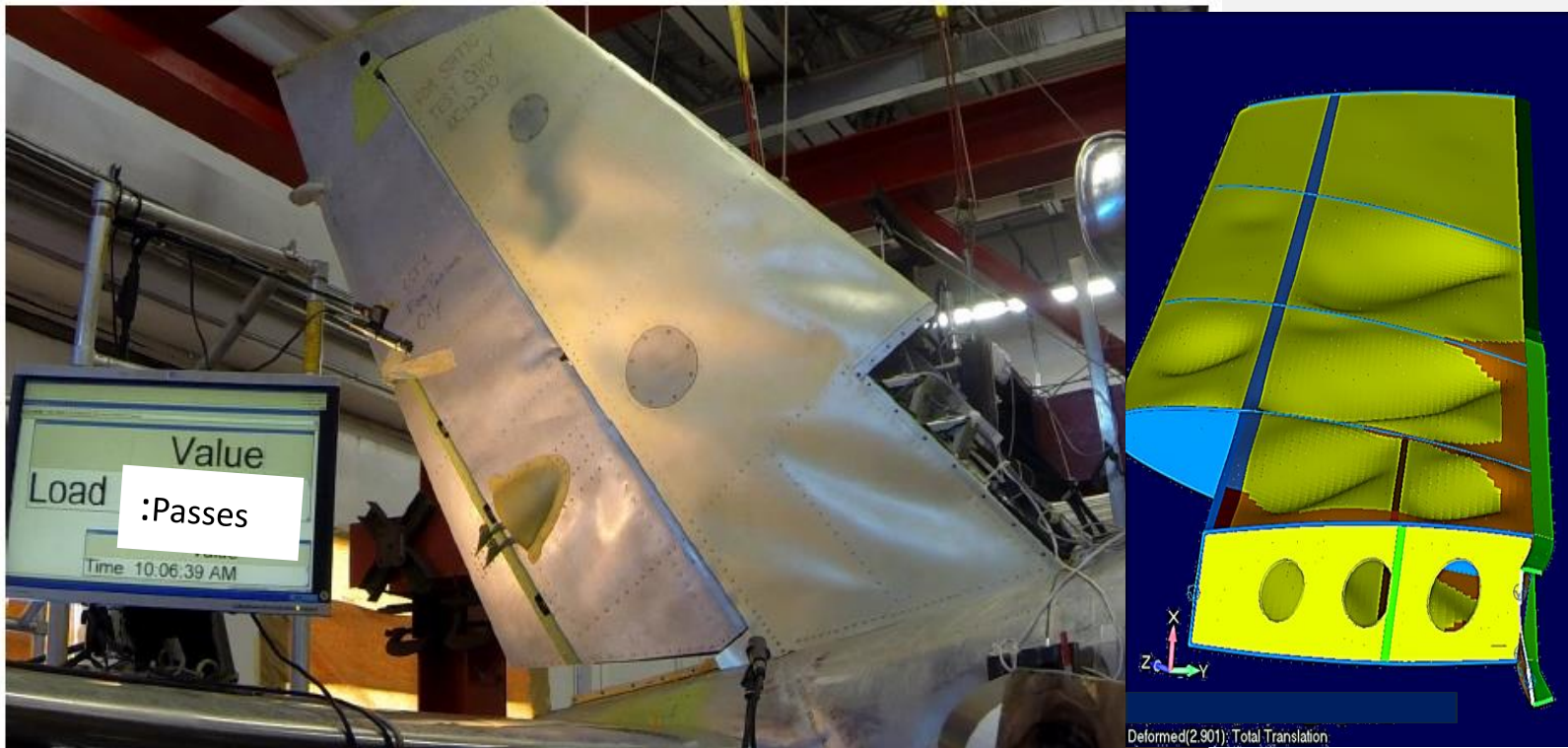
Vertical Stabilizer at load (load level shown is approximate, actual load held was calculated post-test using recorded data)
