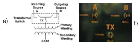
Figure 6. a) Loop switch with ON-OFF radial switch b) Schematic.
