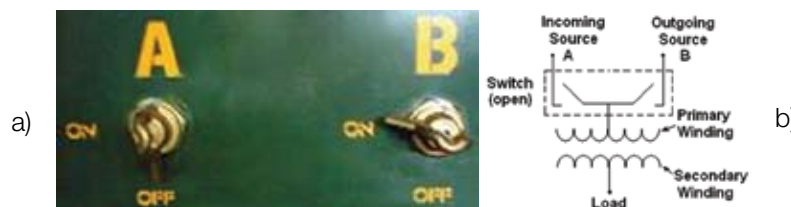
Figure 4. a) Loop Feed Switch b) Schematic of the Loop Feed Switch.
