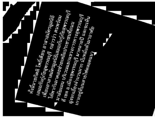
Fig. 3. Output of Locally Adaptive thresholding image after AND filtered and unfiltered grayscale image
