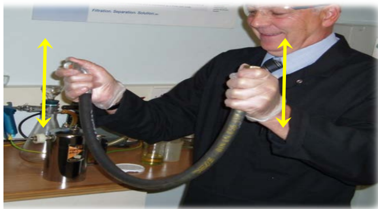
Figure 9 - Agitation (Slosh Test) Extraction Method
