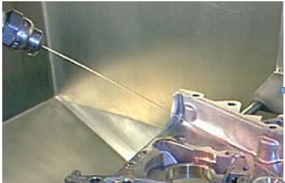
Figure 10 – Pressure Rinse Extraction Method
