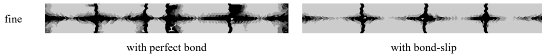
Figure 3.10 External and internal crack pattern in reinforced concrete prism subjected to a tensile load; effect of mesh density when assuming perfect bond or a bond-slip relation. Based on Grassl et al. (2018).
