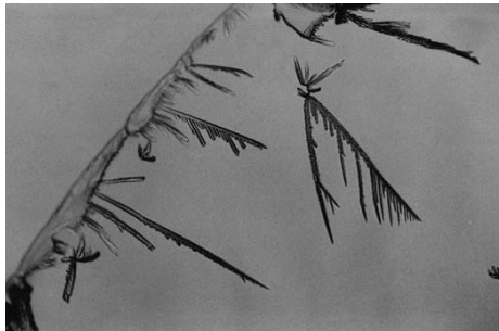
Figure 3. Cocaine and platinic chloride, 100x
