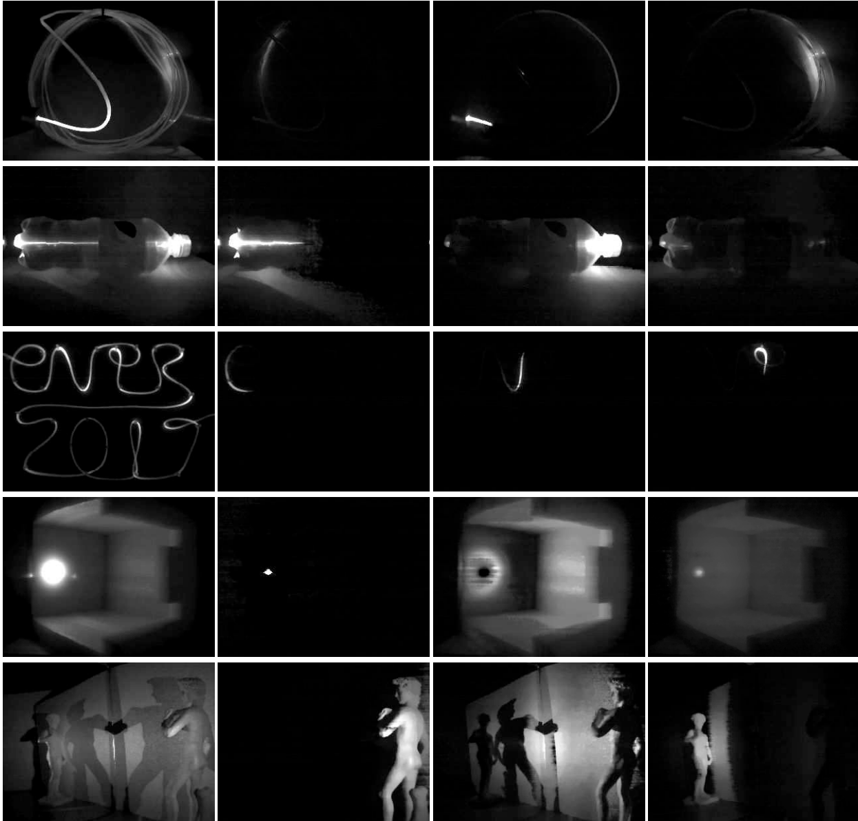
Figure 11. Reconstructed transient images using the Poisson-TV (3D) prior. Column 1: Images of the scene under laser illumination. Each pixel value in this image is the result of integrating the number of photons in a histogram. Column 2-4: Frames from a transient image appearing in chronological order.
