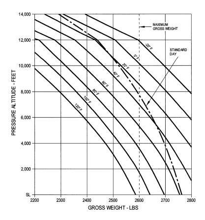
Figure 5-3. Hover Ceiling In-Ground Effect
