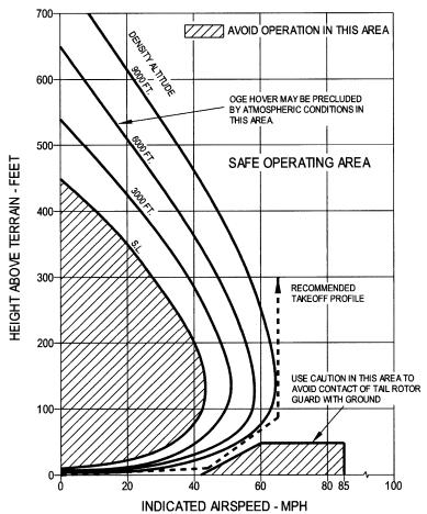
Figure 10-1-5. Height Velocity Diagram
