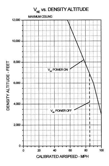
Figure 10-8-1.  $V_{\text{NE}}$  vs. Density Altitude Emergency Float Configuration
