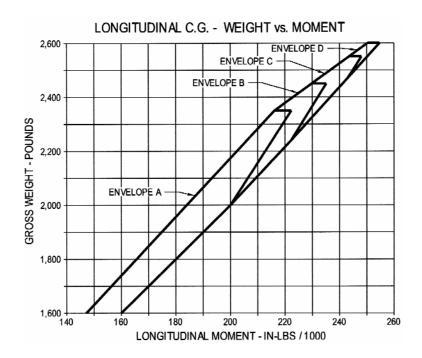
Figure 6-6. Gross Weight vs. Longitudinal Moment
