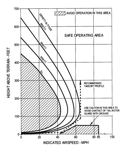
Figure 5-7. Height Velocity Diagram 2600 lb Gross Weight
