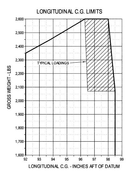
Figure 10-1-6. Gross Weight vs. Longitudinal C.G.
