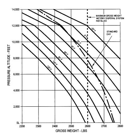
Figure 10-1-3. Hover Ceiling In-Ground Effect
