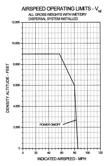
Figure 10-1-1.  $V_{\text{NE}}$  vs. Density Altitude  $V_{\text{NE}}$  Demonstrated at 334 Rotor RPM
