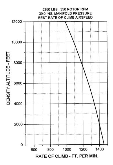
Figure 5-9. Best Rate of Climb Speed Best rate of climb speed varies with altitude 57 MPH IAS at SL decreasing to 48 MPH IAS at 12,000 ft  $H_{\rm d}$ .
