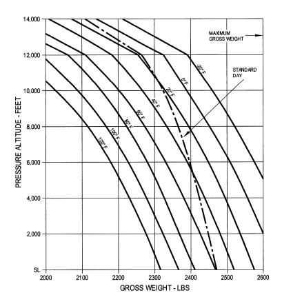
Figure 5-4. Hover Ceiling Out-of-Ground Effect
