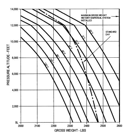
Figure 10-1-4. Hover Ceiling Out-of-Ground Effect
