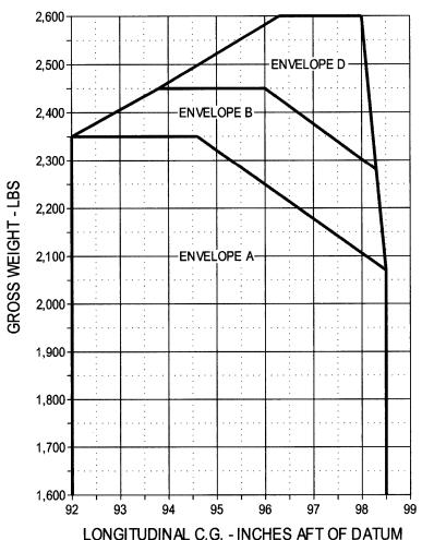
Figure 10-2-3. Longitudinal C.G. Limits
