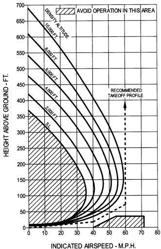
Figure 5-5. Height Velocity Diagram
