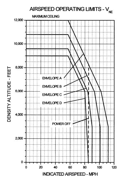
Figure 5-1.  $V_{\text{NE}}$  Variation with Density Altitude
