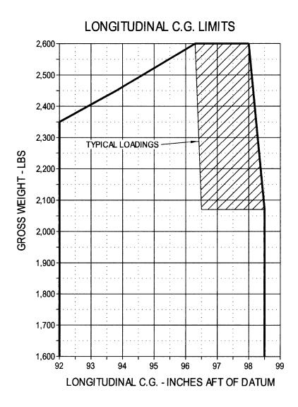
Figure 10-3-1. Longitudinal C.G. Limits
