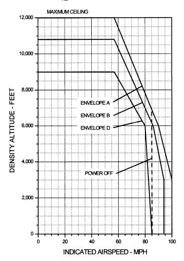
Figure 10-2-1. V<sub>NE</sub> vs. Density Altitude
