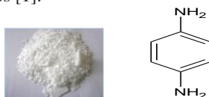
Figure 1: Physical aspect and chemical formula of para-phenylenediamine C_6H_4(NH_2)_2
