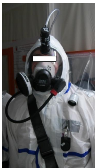
Figure 1. Operator equipped with a modified Vision 3 INRS ® mask enabling assessment of the protection factor.
